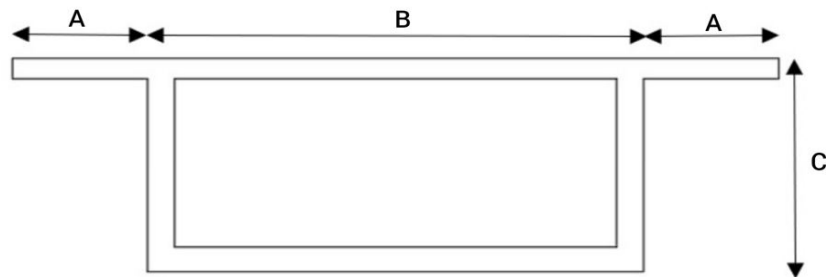
Fig. 1: Cross-section of box girder
